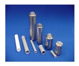
Our Fast Loop filters are constructed from 316L stainless steel. This straight through design is ideal for heavily contaminated systems since the filter element is continuously flushed by the high flow rate stream. Only the low flow (analyzer) stream is filtered, thus maximizing filter element life. Traditional T-type by-pass filters are detailed in Filters for Instrumentation & Analysis.
