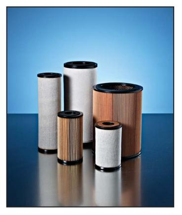
These Facet coalescer cartridges are treated to prevent bacterial growth which could otherwise form on the outer sock. The coalescer cartridges serve the dual function of removing essentially all solids and breaking up emulsions (coalescing) causing large water droplets to form and settle in the sump for periodic draining.
